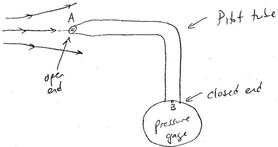
tube is placed parallel to flow
