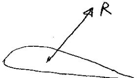
$L$ : lift. Component  $\perp$  to incoming velocity vector (free stream)
