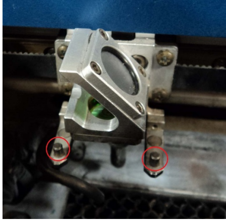
The pins of the laser lens assembly are shown with red circles around them
