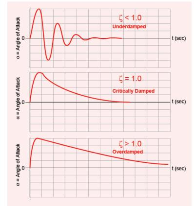
**Figure 1:** The damping ratio tells us how a rocket is going to respond to a disturbance in flight. For example, whether or not it will oscillate.
