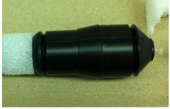
8. Carefully sand the outside of the foam plug glued to the Blow Mold Transition until it slides freely into the Small Payload Tube. Set this assembly aside.
