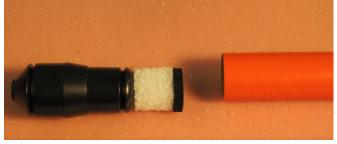
10. Use a generous amount of white glue and glue one of the remaining foam disks to the remaining foam plug. The white glue takes a while to set. The intent is that when assembled, the altimeter will be held in place by the two conductive foam disks.
