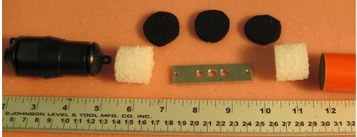
The unassembled pieces of conductive foam and white foam are shown above.
