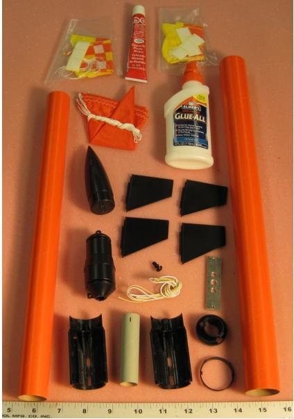
The payload section of the Penetrator must be modified to permit the altimeter to be installed and removed easily. Once installed the altimeter must be held securely and protected against damage. The payload section must also have ventilation holes installed so that the pressure inside the payload section is the same as the free-stream pressure outside the rocket for the altimeter to work properly.
