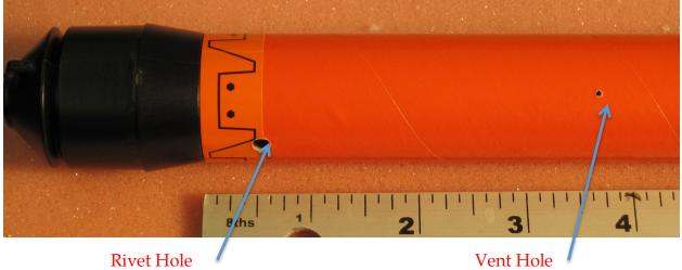
16. Glue the nosecone in place as per Step 4A. of the printed instructions that came with your kit. Put the glue inside the tube, not on the nosecone shoulder. Set the tube with the nosecone pointed down while the glue dries. Do *not* do Step 4 B.
