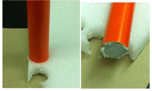
3. Use a 1-in diameter dowel to push the plugs back out of the tube.
