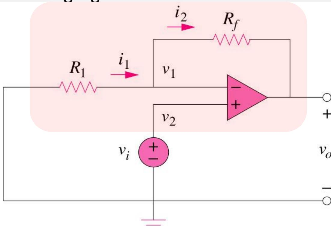
$$v_o = \left(1 + \frac{R_f}{R_1}\right)v_i$$
