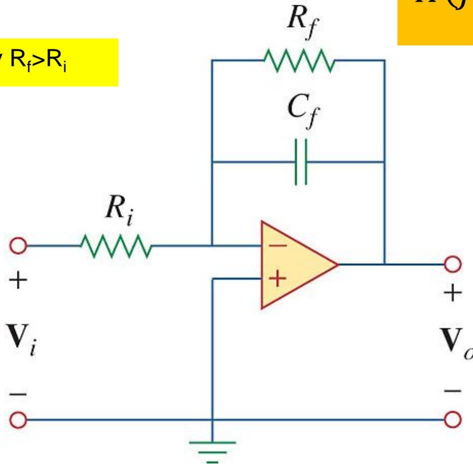
$$H(j\omega) = -\frac{R_f/R_i}{1 + j\omega R_f C_f}$$
