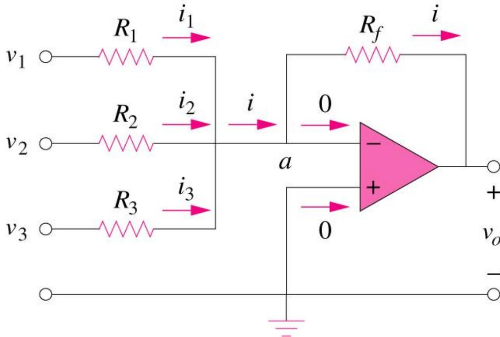
$$v_o = - \left( \frac{R_f}{R_1} v_1 + \frac{R_f}{R_2} v_2 + \frac{R_f}{R_3} v_3 \right)$$
