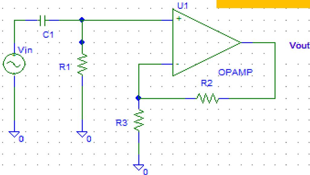
Non-inverting 1<sup>st</sup> order high pass active filter.
