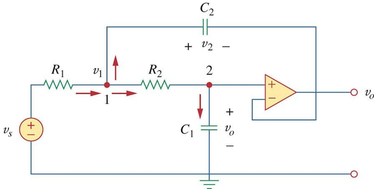
$$H(j\omega) = \frac{1}{1 + j\omega(R_1 + R_2)C_1 - \omega^2 R_1 R_2 C_1 C_2}$$
