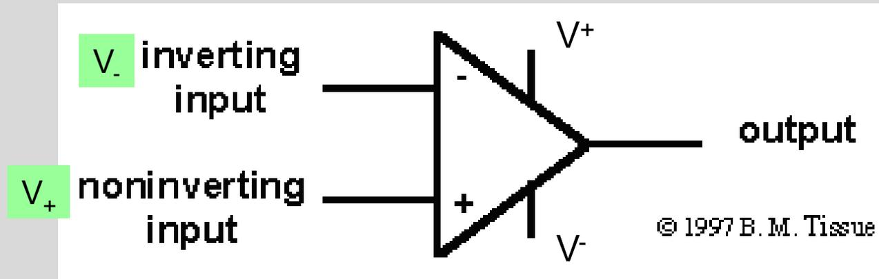
$$(1) v_+ = v_- \quad (2) i_+ = 0, \quad i_- = 0$$
