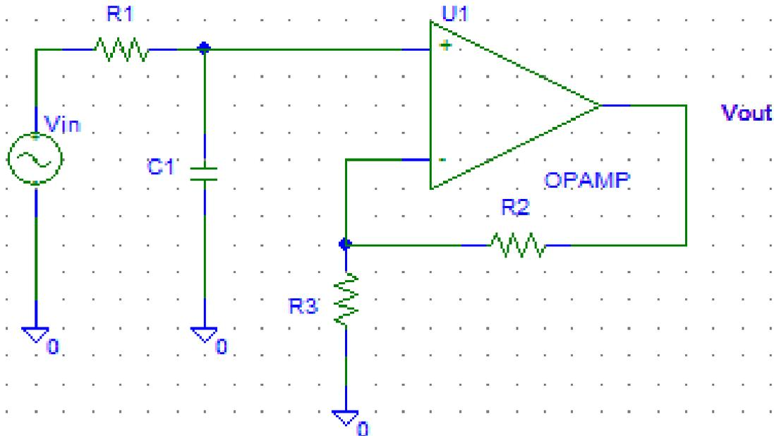
Non-inverting 1<sup>st</sup> order low pass active filter
