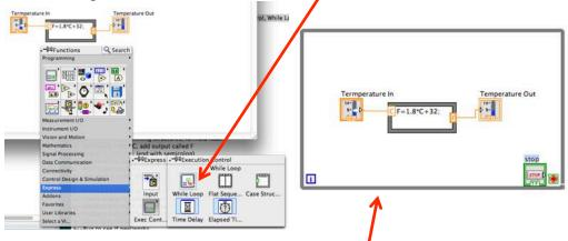
Place the While Loop around the blocks already in the block diagram. You may have to add the stop button if it isn't present. Simply right click the left side of the red circle and select "Create Control".
