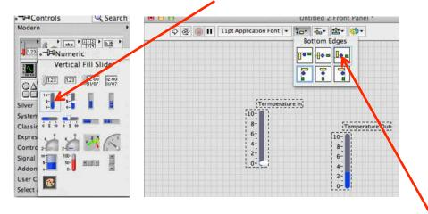
Right Click the front panel, select Numeric->Vertical Fill Slider
