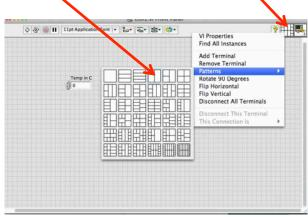
Set the input to the subvi by selecting the left block of the pattern and then selecting the "Temp in C" text field.
