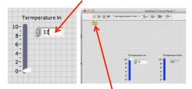
Press the triangle located at top left of pane to RUN. The values of both sliders should now match
