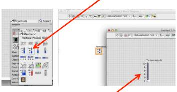
Drag the slider to an exciting place on the panel, rename it "Temperature In" by clicking the text box. Note, the corresponding block that appears in the block diagram.
