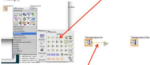
Wire the output of "Temperature In" block to an input to the multiply block.
