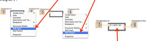
Add the equation into your formula node. Don't forget a semi-colon. Wire it up. RUN the vi and make sure it works.
