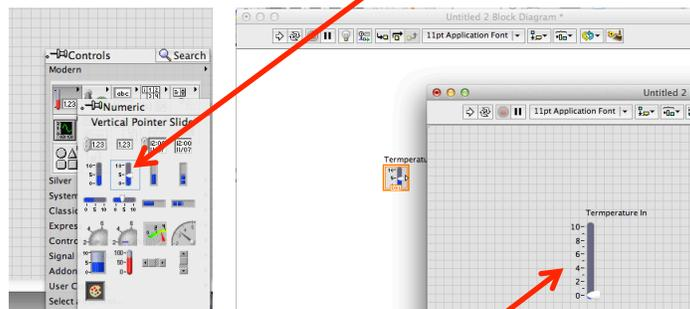
Drag the slider to an exciting place on the panel, rename it by clicking the text box. Note, the corresponding block that appears in the block diagram
