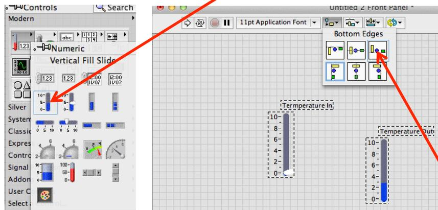
To align the sliders on the front panel, select them both and choose an alignment tool.
