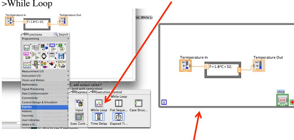
Place the While Loop around the blocks already in the block diagram. Note the Stop button that appears as well as the Loop condition.
