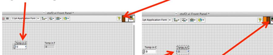
Set the output to the subvi by selecting the right block of the pattern and then selecting the "Temp in F" text field.
