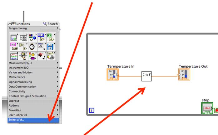
Place and wire up the C to F icon (i.e. your subVI function) in the original block Diagram.
