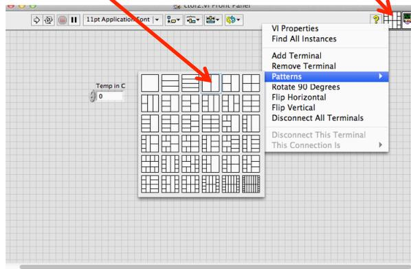
Set the input to the subvi by selecting the left block of the pattern and then selecting the "Temp in C" text field.
