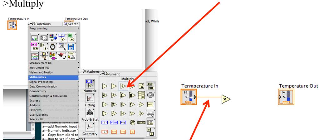
Wire the output of “Temperature In” block to an input to the multiply block.
