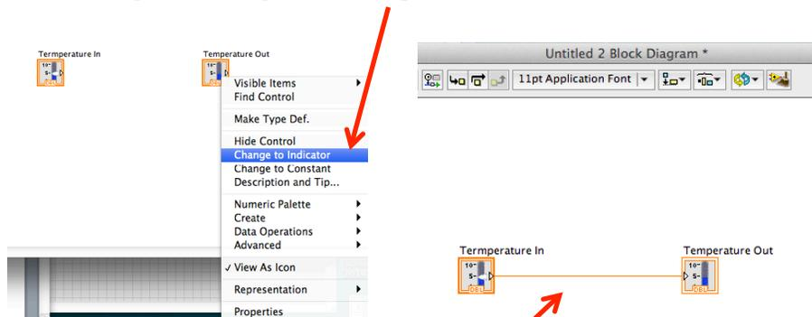
Drag a wire to connect the output from the "Temperature in" block to the input of the "Temperature out" block.
