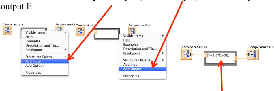
Add the equation into your formula node. Don't forget a semi-colon. Wire it up. RUN the vi and make sure it works.
