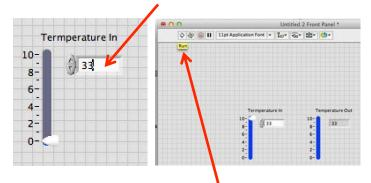
Press the triangle located at top left of pane to RUN. The values of both sliders should now match
