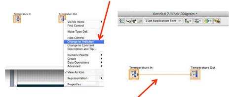
Drag a wire to connect the output from the "Temperature in" block to the input of the "Temperature out" block.
