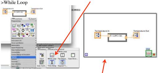
Place the While Loop around the blocks already in the block diagram. You may have to add the stop button if it isn't present. Simply right click the left side of the red circle and select "Create Control".
