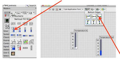
To align the sliders on the front panel, select them both and choose an alignment tool.
