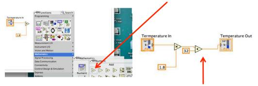
Wire the output of the Multiply block to an input to the Add block.
