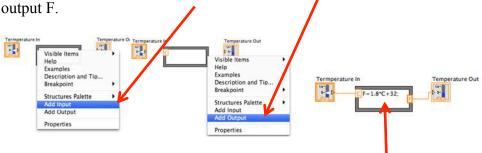
Add the equation into your formula node. Don't forget a semi-colon. Wire it up. RUN the vi and make sure it works.
