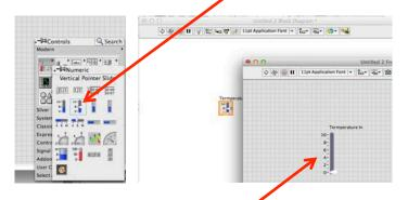
Drag the slider to an exciting place on the panel, rename it "Temperature In" by clicking the text box. Note, the corresponding block that appears in the block diagram.
