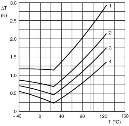
Curves valid for 2.2 to 10 k $\Omega$ Curve 1:  $\Delta R_{25}/R_{25} = 5$  % Curve 2:  $\Delta R_{25}/R_{25} = 3$  % Curve 3:  $\Delta R_{25}/R_{25} = 2$  % Curve 4:  $\Delta R_{25}/R_{25} = 1$  % (for 2381 640 5.... series only)
