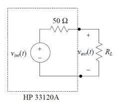
The voltage that will be seen at the output of the signal generator is:
