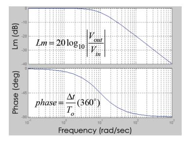
Remember that to make an experimental Bode plot you must measure **both** the output and the input.
