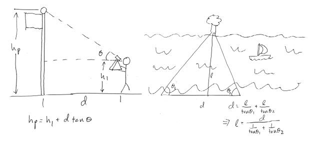
Triangulation is commonly taught as a means to measure the apogee of a model rocket in K-12 rocketry events. The distance from the launch stand to the inclinometer is measured and then the angle when the rocket is at apogee is measured. The major assumption is that the rocket flies straight up from the launch stand, which is rarely the case. The resultant altitude calculations can be way off.
