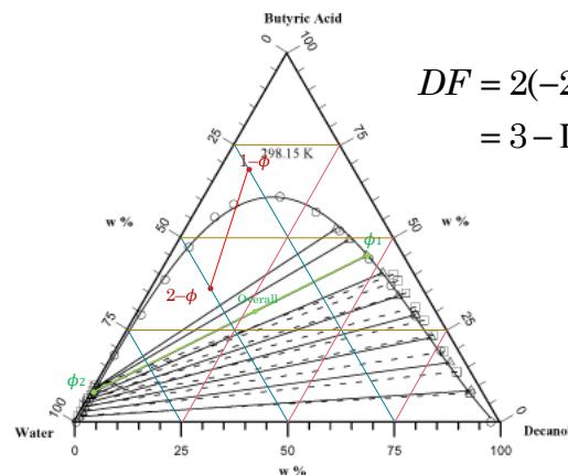
Figure 2: Ternary diagram for LLE of water (1) + butyric acid (2) + decanol (3) at 298.15 K; —○— experimental solubility curve; —Δ— experimental tie lines; ---□--- calculated (UNIFAC method) tie lines.
