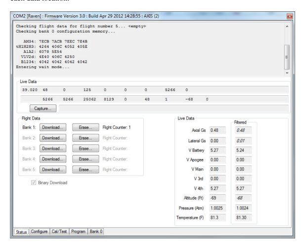
In the example above, 1 out of the 5 flight banks are full. The most recent flight (#1) is located in bank 1.
