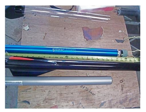
Close up reveals the magic number is 24in. for the edge of coupler. I will use rivets to hold in the assembly, but not drilled through the coupler, too hard to locate them. Drilled above the coupler I want the coupler removable to clean and also bang out motors [friction fitted] with a stick. Insert the assembly push past the rivet holes. Insert rivets Pull assembly up tight to rivet so there is no slack.
