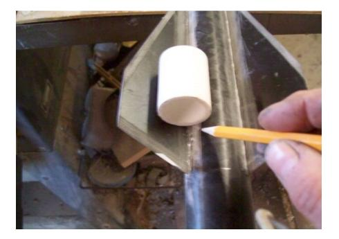
Lay tape ,butted to marks front to back. check alignment with tool and adjust tape. The closer to where the tool hits tube and fin, the less sanding will be needed to attain great fillets!
