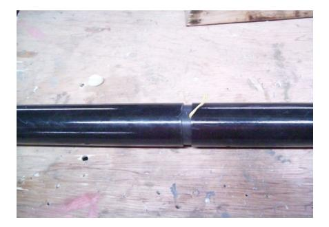
Drill small [1/16] vent hole in the middle of both airframe sections to bleed off internal pressure during flight.
