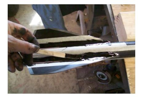
Spreading the epoxy into the V-groove as evenly as possible. Level out the epoxy as best you can. Makes it easier to pull the fillet later.
