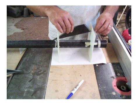
With one hand holding fin in front of guide, use other to grab fin between guides. Slide fin through rear guide and position above the line.
