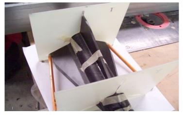
Using a 1in. section of PVC pipe for my tool to pull out fillets, first use it as the guide for placement of masking tape.
