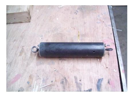
Av-bay held in by 2 rivets opposite on another. 2 tiny vents between them. Positioned 1  $\frac{1}{2}$  from edge of airframe. 5/32 bit used for drilling rivet holes.
