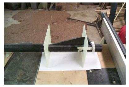
Black epoxy is mixed 5.5 resin to 1 part hardener. This stuff is pretty gooey and a tad hard to work with if you've never used it before. I use a scale to weigh it. It does flow out beautifully however. For tacking the fins, I use JB Weld, either will work fine. I just did not want to measure and mix such a small amount of the high temp stuff.
