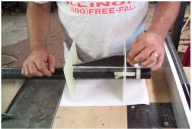
If guide holds the fins a tad loosely you can improvise by using pencils to wedge them in place while curing so they can not move. A little more tape to hold things in place.
