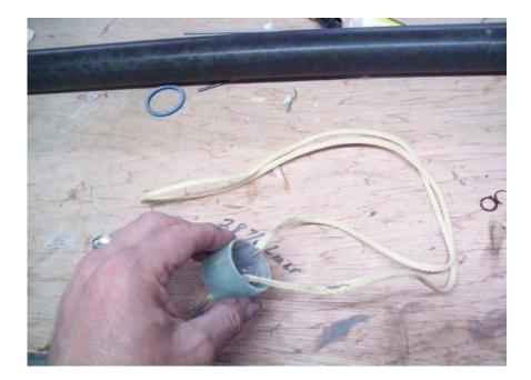
Proper placement of recovery harness is just above the largest motor case you will fly/fit into the rocket.
