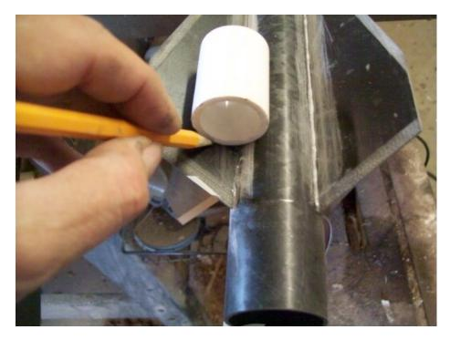
Mark where tool edge hits tube. Mark at front and rear of tube.
