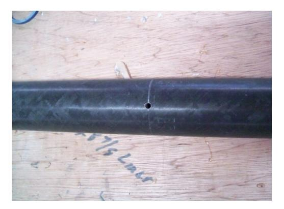
When prepping, just fish wire through hole in av-bay, or connect switch.
