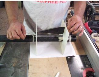
Working from rear to front, push fin down into position. Not to hard but firmly, you do not want to push out all the epoxy from under the fin. Rotate guide and repeat for 2nd and 3rd fins. Or just do one. Set aside to cure.
