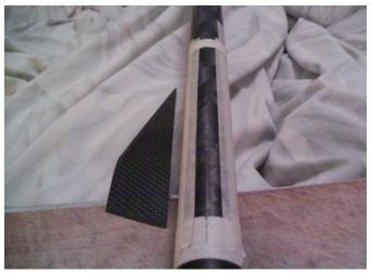
Fins come beveled, so you only need to sand the root for glue adhesion and fillets.
