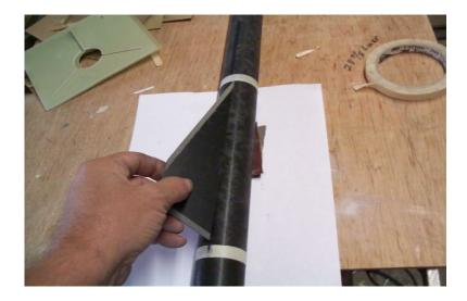
Rough up the surface on each side of line with 60-80 grit sandpaper for fillet adhesion.
