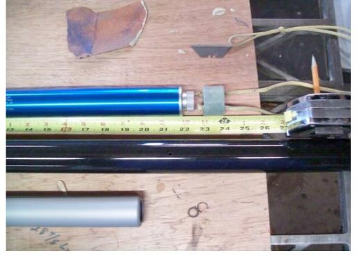
This is what it would look like in proper position internally, rivet in place. 2 rivets 180 degrees opposite on airframe. I'm sure the altitude junkies will use a glue in technique, or flush mount screws or some type aero-dynamic trickery to squeeze out the last bit of performance.
