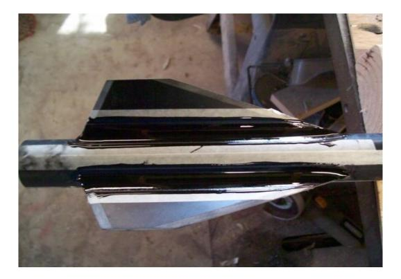
Remove tape after 15-20 minutes, before epoxy cures. If you wait till full cure it will be very difficult. Finished fillets.
