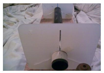
Prep tube & guides by pre-fitting a fin in place to show where they should be located. I had to shim the tube a little with tape to get a snug fit, then taped guides in place.
