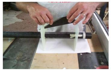
Keep front of fin up and lower back onto line, and into proper position.
