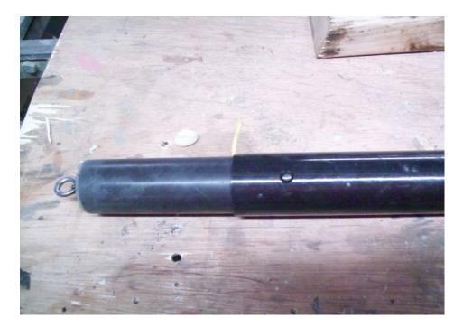
Assemble, push the 2 airframe sections together and drill hole [5/32] centered on joint.
