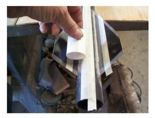
Use 15 grams of resin to 3 of hardener for each set of fillets [2 fins] .
