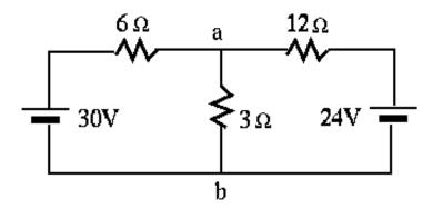
**Solution:** move two voltage sources to left, and 3  $\Omega$  resistor to the right as load find equivalent voltage Vo and internal resistance and Ro.
