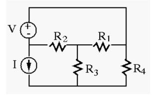
Alternatively, rearrange the components as shown in the figure above and assume the node between the current and voltage sources is grounded  $V_2 = 0$ , then  $V_3 = 50V$ , and denote previous ground
