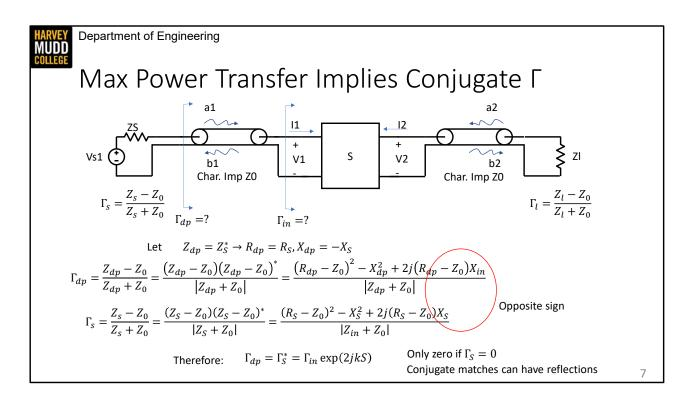
Let's start with a standard picture of a S parameter network, but note that I've added an unusual reflection coefficient on the left called Gamma\_dp. This is the implied reflection coefficient off the driving point of the left transmission line. We usually think about the driving point impedance, Zdp, but Z and Gamma map to one another 1 for 1, so we can define a Gamma\_dp if we feel like it. We're curious about what Gamma\_dp will be if we are trying to achieve maximum power transfer.
