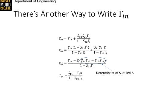
There's one common alternate form for Gamma\_in that we need to derive.
