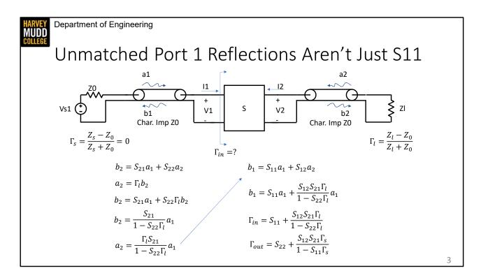
I've drawn a two-port network here that has a mismatched load. That means that we need to define a reflection coefficient off the load, and we have done so in the form of Gamma\_I. The source is matched in this example. We're curious what a reflection off the input port looks like now that we'll see some additional power into port two from load reflections. We'll call the effective reflection coefficient Gamma\_in.
