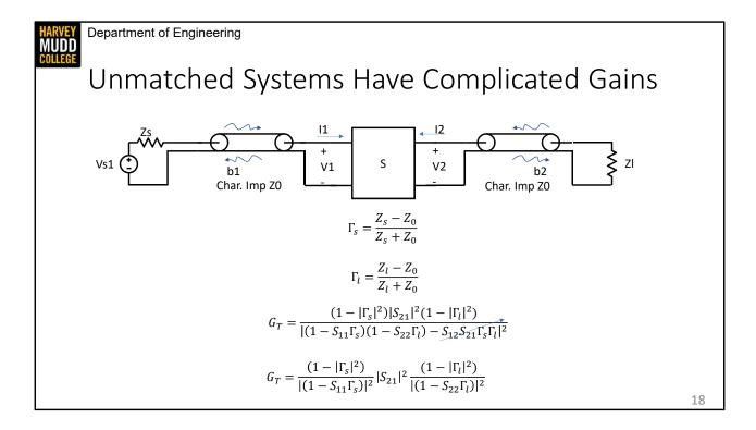
We can still find power gains if we relax the constraint that the source and load impedances are matched. I've defined reflection coefficients off of the source and the load on this slide, and I've also given you a transducer power gain with no justification. The math is uglier, but you can see that this reduces to the magnitude of S21 squared if Gamma\_s and Gamma\_l are zero. Great!
