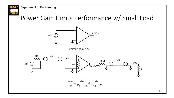
One of the first things to discuss is the need for power gains at all. You've used amplifiers before, and we've mostly thought of a voltage source driving them, and the amplifier providing some voltage gain to that voltage source. For instance, this is probably how your learned to think about op-amps. Voltage gains seemed to work great up until now.
