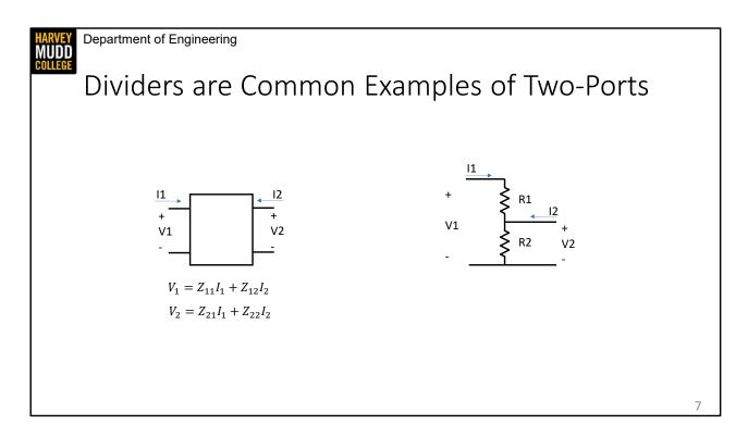
The left side of this slide shows a generic two port while the right side shows a divider, which is a specific example of a two port network. I've drawn ports 1 and 2 on the divider so that we can make a comparison to the generic two port throughout this video. Note that we define all the currents in a two port as pointing into the network for consistency, and we see that in both the generic two port and the divider.
