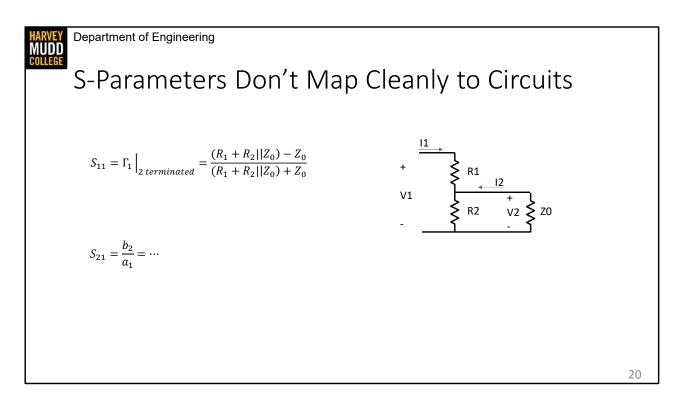
While S-parameters are easy to measure, we're going to find they are tough to analyze. If I was trying to find the S-parameters of our divider, I could start by attaching Z0 to port 2. Making that connection ignores the transmission line connecting port 2 to the termination, but this is OK because the driving point impedance of a transmission line with a matched load is always Z0 anyway. So we can find reflection coefficient of this structure from the Thevenin impedance of the load.
