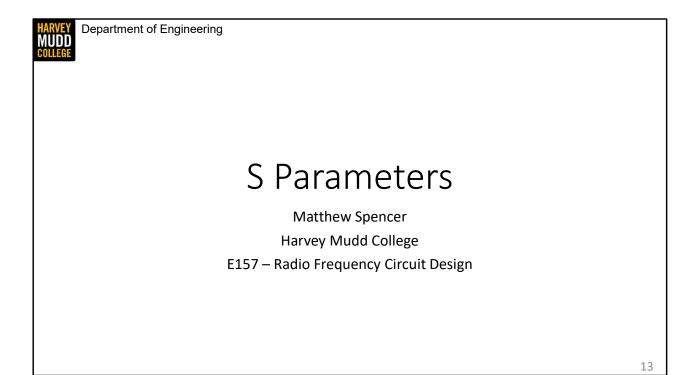
In this video we're going to learn about yet another set of linear parameters called S parameters, where the S is short for scattering. Though we've already got two perfectly good sets of linear network parameters – Y and Z parameters – S parameters are important because they're easy to measure at high frequency. Accordingly, many types of test equipment report S parameter values as their outputs.
