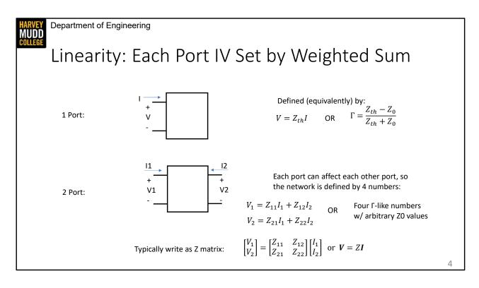
We'll start making our formalism for two port networks by looking closely at one port networks. I've drawn an example one port here, and it has a pair of port variables V and I, and I is defined as positive going into the port. As long as the circuit inside the one port is linear and passive, we can describe the relation between V and I using a Thevenin impedance. Or, equivalently, we could specify a reflection coefficient for the port, which is a one-to-one function of the impedance.
