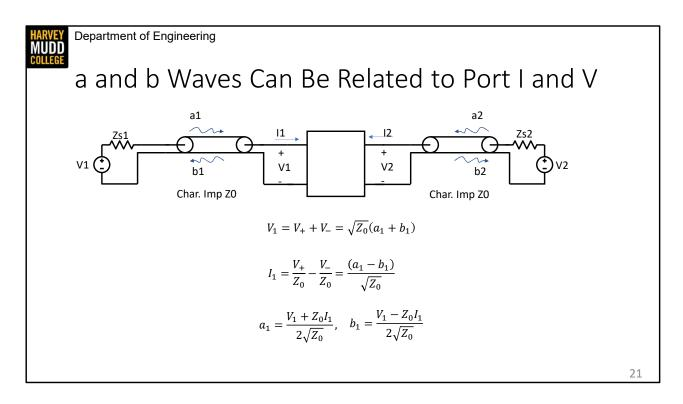
However, we know the port voltages and currents are given by sums of voltage waves and differences of current waves from our earlier study of transmission lines. CLICK That means we can write a1 and b1 in terms of V1 and I1 by adding and subtracting the V1 and I1 equations in the first two lines.
