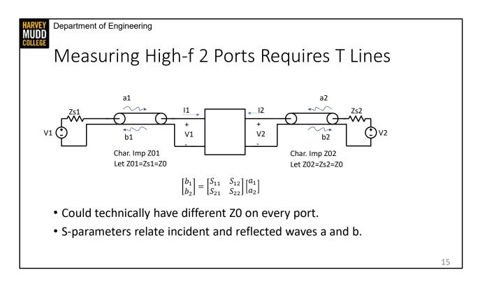
S parameters fix these problems by bolting a pair of transmission lines to the ports of the two port. These transmission lines could technically each have different characteristic impedances, and they could each be driven by different source impedances, but we're going to assume that everything is matched to a value Z0 for now.
