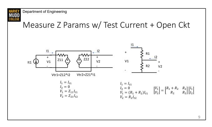
Now that we have an equivalent circuit, we can think about how to measure or calculate the Z parameters for it.
