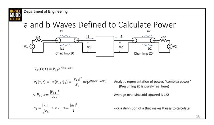
The a and b amplitudes are defined in a special way that makes the calculation of power flow in the system easier.
