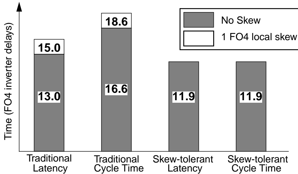
Figure 2-10 Simulated latency and cycle time of adder self-bypass
