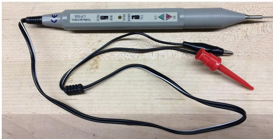
Figure 4: Wavetek Logic Probe
