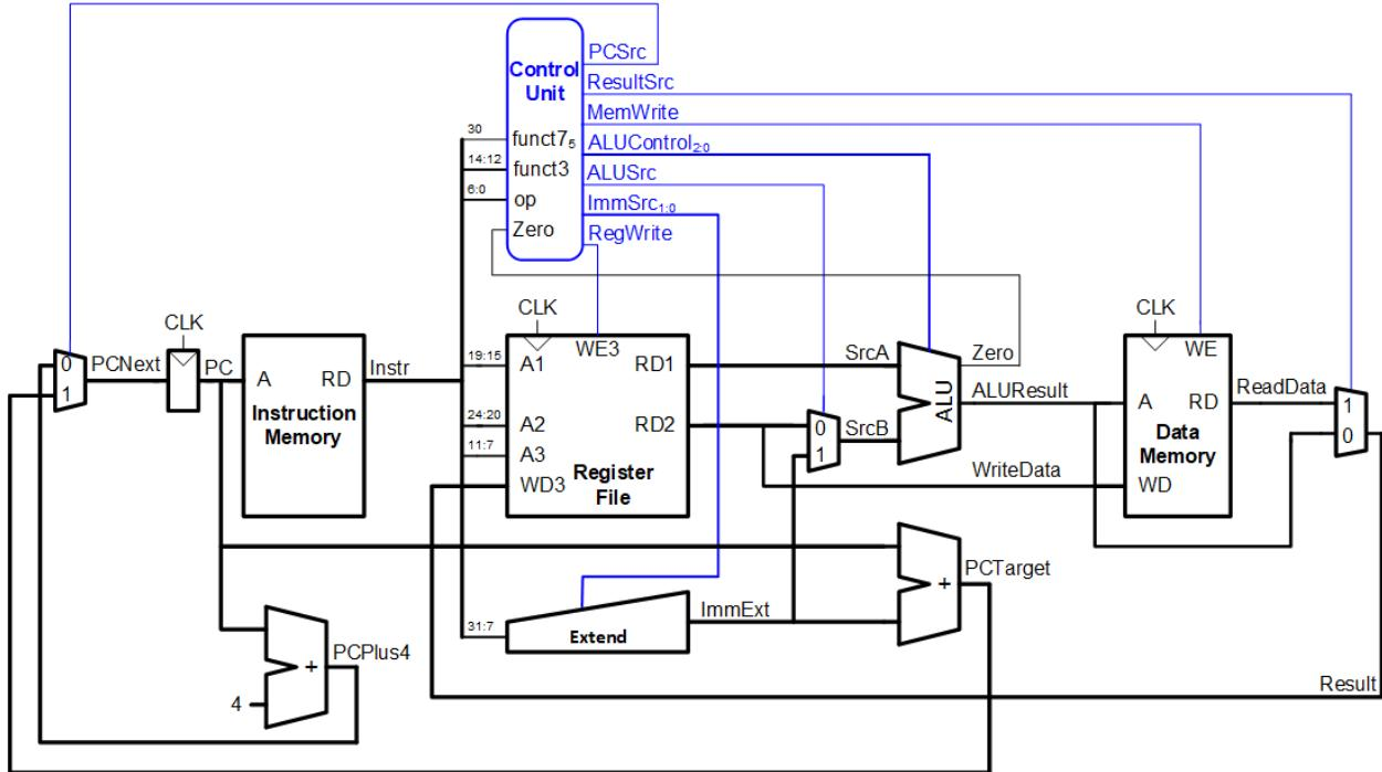
Note: To support JAL, extend the Result mux to 3 inputs, as shown in Fig 7.15 but not important for this problem.
