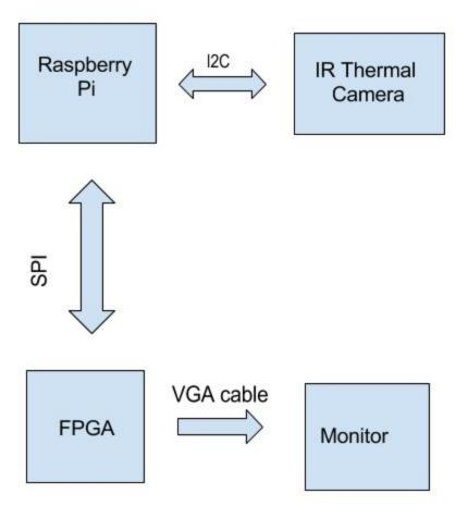
Figure 1. Block diagram of Infrared Thermography system
