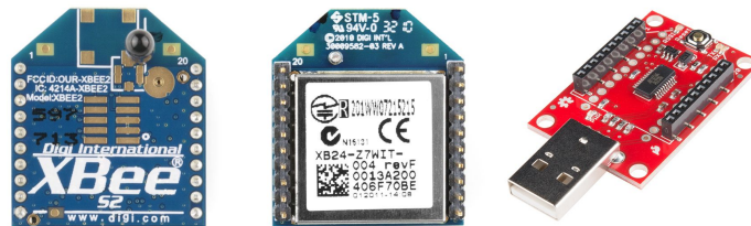
Figure 3. Front (left) and back (middle) of an XBee module. USB adapter board (right) for XBee.
