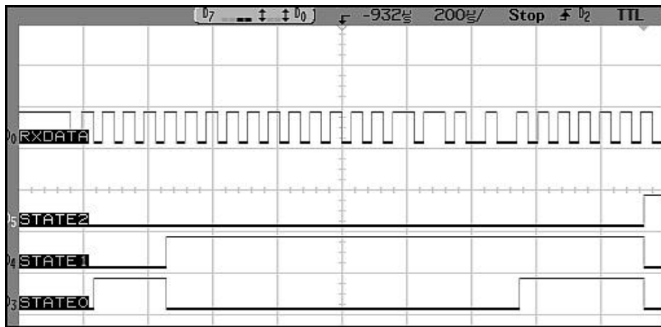
Figure 3. Message Header | A series of 32 sub-bits followed by a data word alignment.
