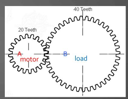
• Gear ratio:  $\omega \downarrow B / \omega \downarrow A = N \downarrow A / N \downarrow B$
