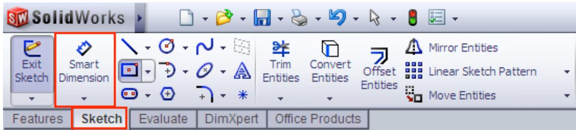
Click on the rectangle's left side, move the cursor a bit to the left, and click again to place the dimension on the sketch. At this point, a window should pop up allow you to set the dimension. We want the rectangle to be 3" by 5", so enter 3 in the window and click the check box.
