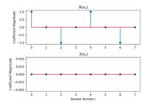
Set f =2 Hz and  $f_s$ =8 Hz. So, this means that we have 4 samples per period of the sinusoid. x[n] = [1,0,-1,0,1,0,-1,0]
