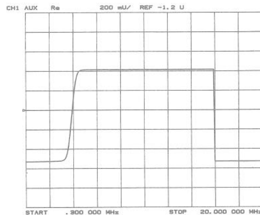
Figure 11. Node 18 IF Det 2N, IF Detector After 3 MHz Filter.
