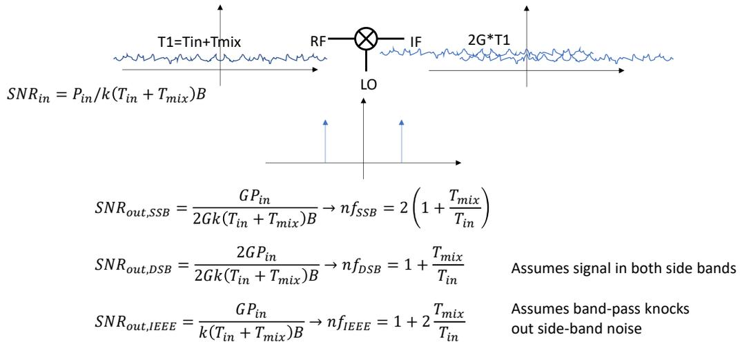
To analyze the noise behavior of a mixer, we're going to imagine that we have noise with a temperature  $T_1$  at the input, which represents a combination of the input noise temperature and the mixer noise temperature. We're going to get two copies of the input noise spectrum at the output, one from the positive LO sinusoid and one from the negative LO sinusoid, that are both scaled by the conversion gain. Getting multiple copies of noise like this is called noise folding.
