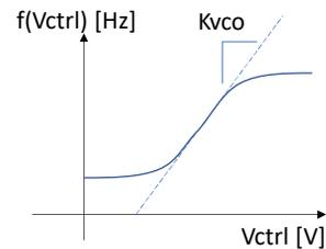
Voltage controlled oscillators are elements that take a relatively slow varying input called the control voltage and produce an output sinusoid whose frequency depends on the control voltage, which I've indicated with the notation  $f(V_{ctrl})$ , to indicate it's some function. The amplitude is set by the oscillator, and generally not controllable.
