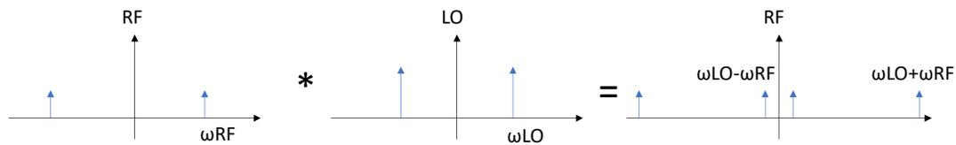
I've pictured mixers in their two common configurations here. There are three ports on a mixer, usually labeled RF, IF and LO. These stand for radio frequency, intermediate frequency and local oscillator. Regardless of whether RF is the input and IF is the output or IF is the input and RF is the output, the mixer does the same thing, which is multiply the input signal by LO. To do this, the mixer generally relies on LO being a very large signal.
