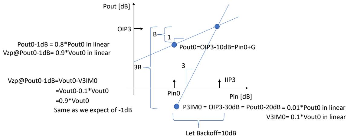
Because the relation between P-1dB and IIP3 is so important, we're going to show another way to find it. We can also use our backoff calculation to show that P-1dB is 10dB below IIP3. We do that by letting our backoff be 10dB, and then showing that the third order intermodulation power would reduce the first order power by 1dB.
