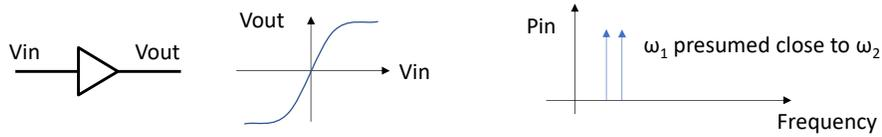
$$V_{out}(t) = a_1 V_{in}(t) + a_2 V_{in}^2(t) + a_3 V_{in}^3(t) + \dots \quad \text{Let } V_{in}(t) = V_1 \cos(\omega_1 t) + V_2 \cos(\omega_2 t)$$
