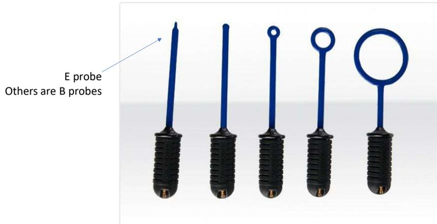
One way that we measure electric and magnetic fields is by taking advantage of their coupling behavior. I've included a picture of a set of near field probes on this slide. The left most probe measures E field, and it looks like a little stick that you could put in a existing capacitive field. The remaining probes are loops of various sizes that measure B fields. Bigger loops are more sensitive, but less area specific.
