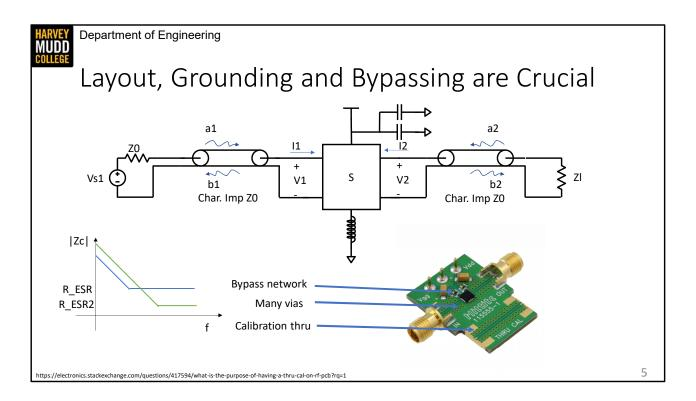
Though most of these videos are going to focus on modeling input and output reflections, there is another source of instability that is much more common. That source of instability is called supply coupling, and it occurs when a two-port network's connection to the power supply has high impedance. This means the power supply voltage can fluctuate during the two-port's operation, which is a parasitic and potentially unstable feedback loop.
