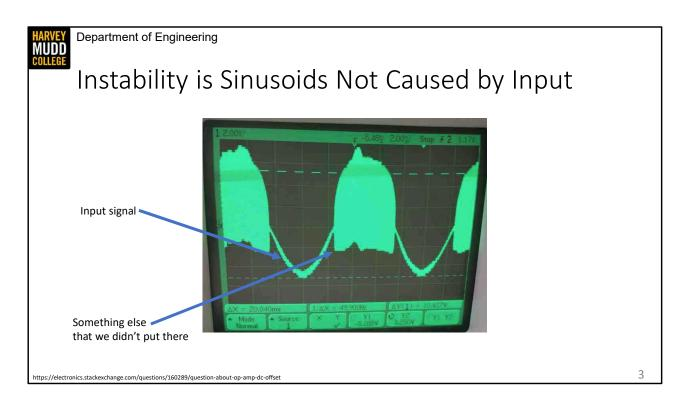
And we need to start by defining what instability is. You may have run into definitions of stability like "Bounded Input Bounded Output" or BIBO in linear systems classes, but I find those definitions are insufficient to circuits. The definitions struggle because all circuits are non-linear eventually; only a precious few circuits can make voltages outside of their power rails. That means all outputs are going to be bounded regardless of input, so BIBO loses some of its charm.
