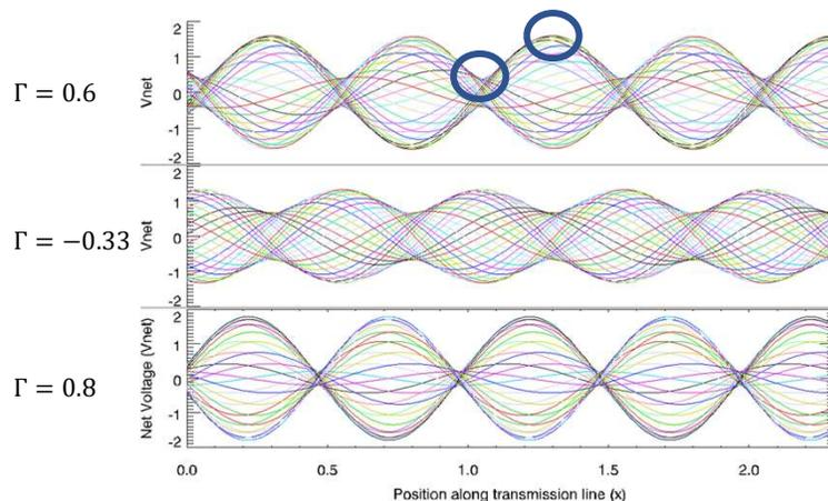
$$|V(x, t)| = V_{zp} \left| \frac{Z_0}{Z_s + Z_0} \right| |1 + \Gamma e^{-2jkx}|$$
