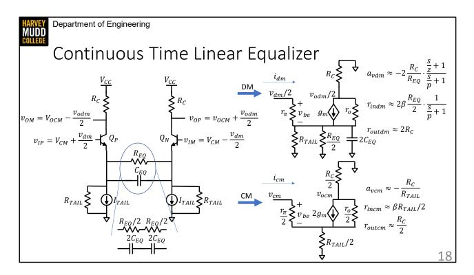
This circuit, called a continuous time linear equalizer, is somewhat trickier than the last one.
