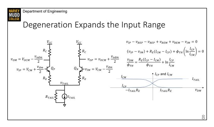
The narrow input range of emitter coupled pairs is annoying, but degeneration can increase it. I've drawn an emitter coupled pair with emitter degeneration here.
