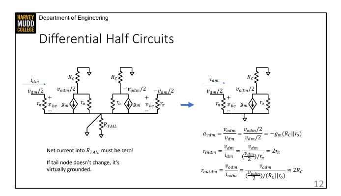
We're going to look at purely differential small signal inputs first, and that's going to result in us drawing something called the differential half-circuit.
