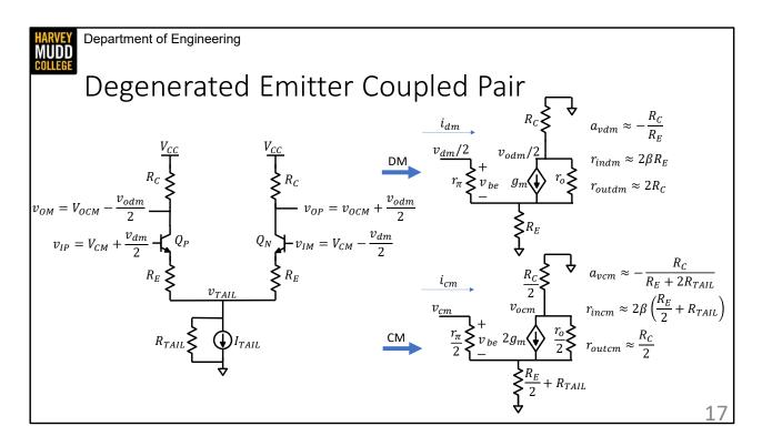
I've drawn an emitter coupled pair with degeneration on the left. Pause the video and find the common mode and differential mode half circuits, then calculate gain, input impedance and output impedance for both the common mode and differential circuits.
