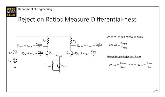
When we build differential amplifiers we usually want them to be sensitive to differential signals and insensitive to common mode signals. Amplifiers have a few figures of merit that help us measure how well we've done in that goal.
