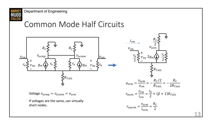
The common mode half circuit has to be analyzed a bit differently from the differential half circuit.
