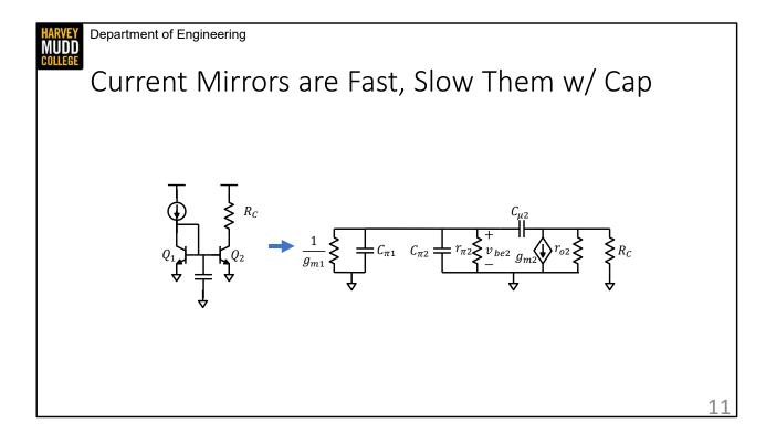
First, current mirrors are quite fast. That's mostly because Q1 looks like 1/gm, which means Cpi1 and Cpi2 see small impedances. Something similar is going to be true of most mirror topologies because a diode connected device is a crucial part of a mirror.
