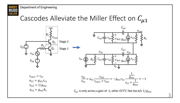
I've included a cascode amplifier on this slide along with a small-signal dynamic model that represents it.
