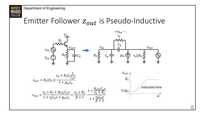
Finally, it's worth noting that the output impedance of an emitter follower appears inductive over some frequencies. I've copied the emitter follower small signal model here, adding my test source at the output and a source resistance at the input. Note that the source could be any impedance in general, but we'll confine ourselves to analyzing a resistance for now.
