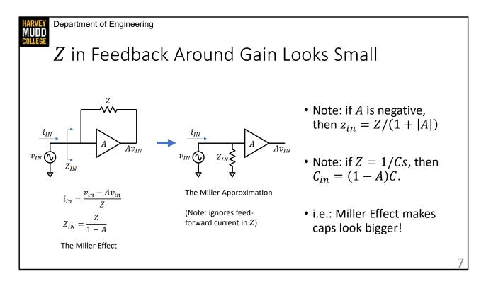
We're going to talk about a circuit behavior called the Miller Effect, and it's easiest to see the Miller Effect in action using this super simplified, single-ended, ideal amplifier. We're curious how having this impedance Z in feedback around the amplifier affects the amplifier's input impedance. Note that the input impedance would be infinite if we were just looking into a perfect amplifier, so this Z is almost guaranteed to lower the input impedance.
