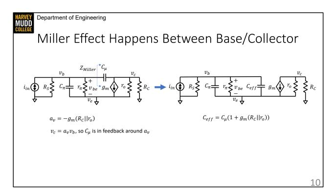
I've copied our model for the dynamic common emitter here, and we're going to see if we can make it simpler using the Miller Approximation.
