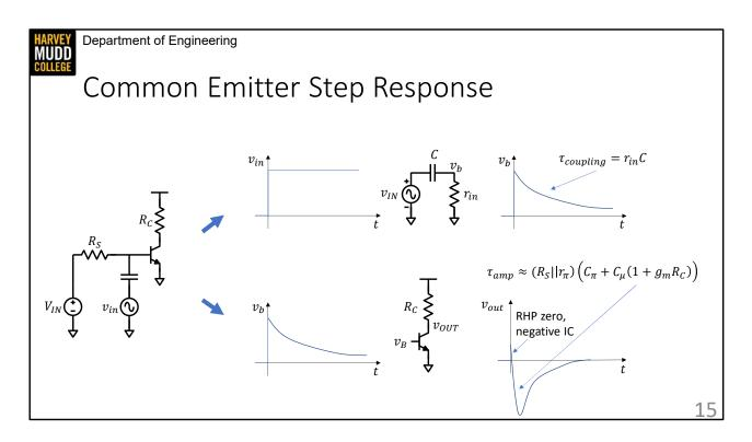
That's a bit abstract, but we can take a quick look at how it plays out in a common emitter. One important and common situation is where we're trying to measure the step response of an AC coupled amplifier like the one I've drawn on the left.
