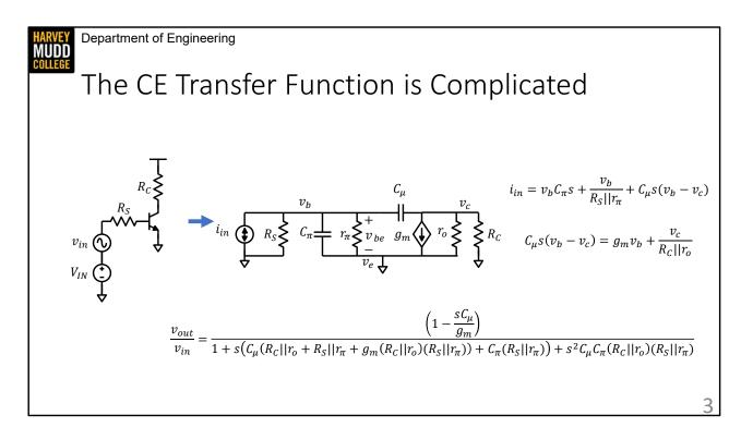
I've drawn a common emitter on the left here and put its dynamic small signal model in the center of the slide. I took an unusual step when I made the small signal model, which was converting the input voltage source into an input current source. This just saves us a bit of algebra.
