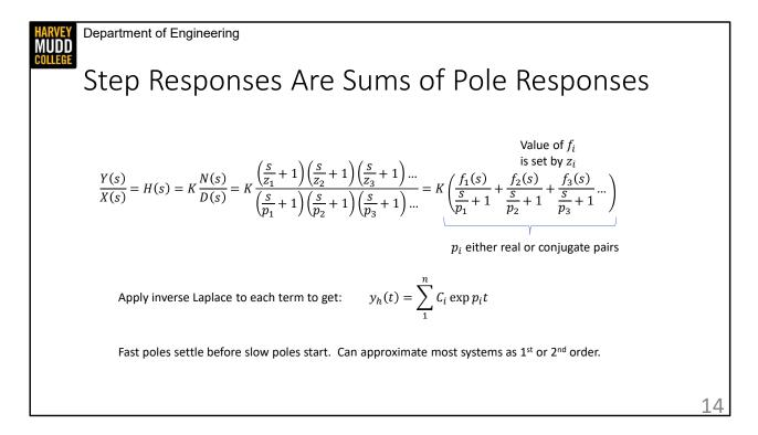
We often focus on the frequency domain when we're doing amplifier design because using impedances make frequency domain analysis so easy. However, the step response performance of amplifiers can be more important than their bandwidth in some applications.
