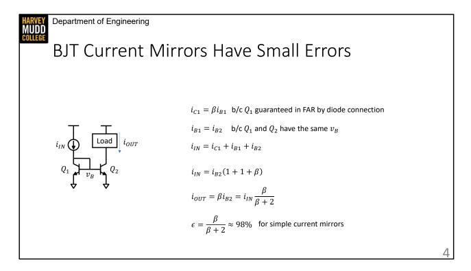
Alright, back to relating iC1, which is equal to iC2, to i\_IN.
