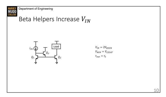
Calculating the other current mirror parameters for this current mirror is pretty straightforward. Pause the video and try to find VIN, VMIN and rout.
