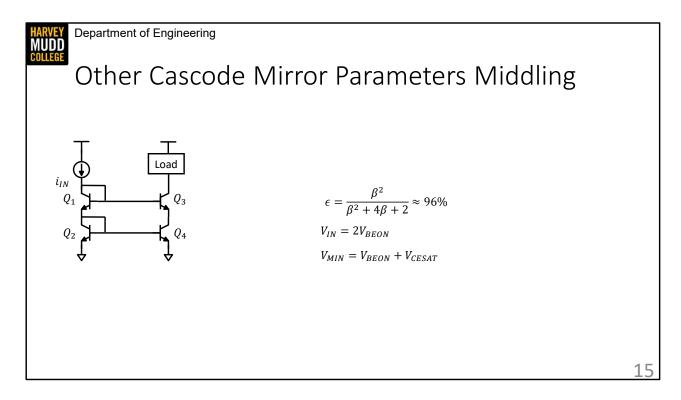
Epsilon is also involved for a cascode amplifier so I've just included it on this slide. It's worth noting that the error is pretty middling. The other cascode amplifier parameters are easier to find. Pause the video and find VIN and VMIN.
