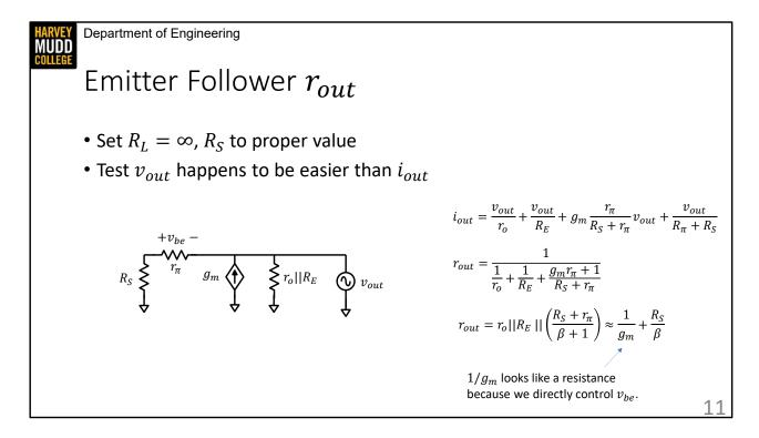
Finally, we're going to find rout of the emitter follower. Our rout test conditions are an infinite load resistance, so it doesn't steal any current from our output, and an RS that is normal for the amplifier. We're choosing to use a test voltage source for this analysis because it makes our life easier. Pause the video and try to find rout.
