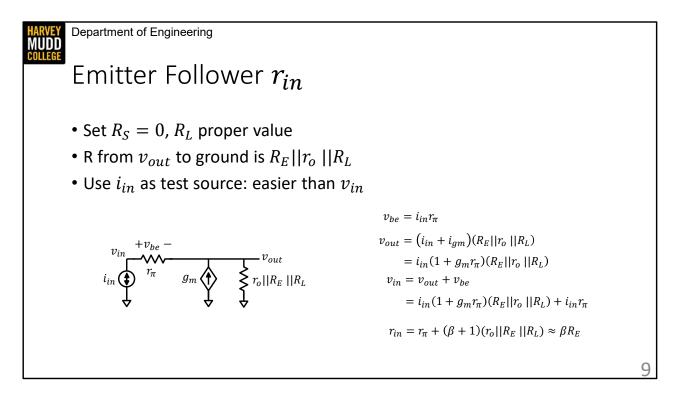
We set up our analysis to find rin by remembering the test conditions we use for rin. We set RS to zero so it doesn't add to the rin that we calculate, and we set RL to an appropriate value so that any feedback effects in our amplifier get captured by rin. Because RL would be connected between vout and ground, it just falls in parallel with our ro||RE resistor from the previous page.
