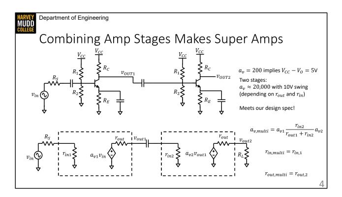
OK, that's rough, but what if we stuck two common emitter amplifiers together? Maybe this would produce the gain we needed without needing a crazy VCC value. It certainly looks like a nice idea, but the idea of re-analyzing some big structure with two small signal models inside of it seems like a pain. Notice that I've coupled the amplifiers together with a capacitor, so they can each have different DC bias points.
