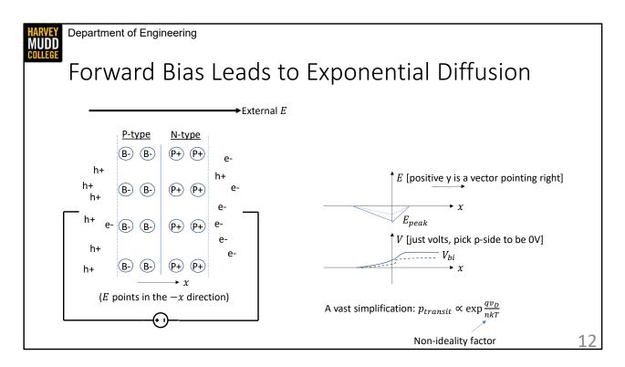
Apply a voltage to the diode unbalances the two currents by changing the total electric field in the PN junction. This process is complicated, and we're painting a vastly simplified picture on this slide for expediency's sake.
