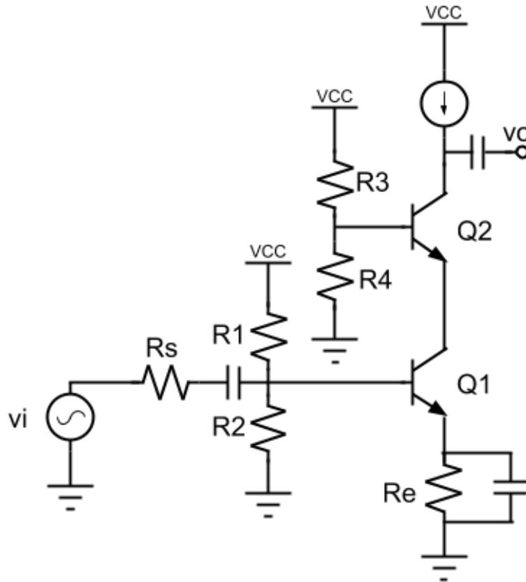
Figure 1: A sample design for a cascode amplifier.
