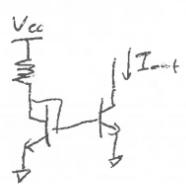
$$\begin{aligned} S_{V_{cc}}^{I_{out}} &= \frac{V_{cc}}{I_{out}} \cdot \frac{\partial}{\partial V_{cc}} \left[ \left( \frac{\beta}{\beta+2} \right) \cdot \left( \frac{V_{cc} - V_{be,01}}{R} \right) \right] \\ &= \frac{\beta}{\beta+2} \cdot \frac{V_{cc}}{R} \\ &\quad \left( \frac{\beta}{\beta+2} \right) \left( \frac{V_{cc} - V_{be,01}}{R} \right) \end{aligned}$$
