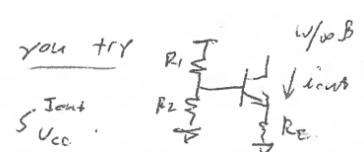
$$\frac{\partial I_{outb}}{\partial V_{cc}} = \frac{R_2}{R_E} \cdot \frac{V_{cc}}{R_1 + R_2}$$
