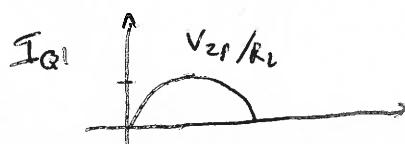
$$P_{\text{Supply}} = V_{ce} \cdot I_{\text{Supply}}$$
