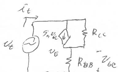
$$i_t = g_m v_{BE} + \frac{v_t - v_E}{R_{cc}}$$
