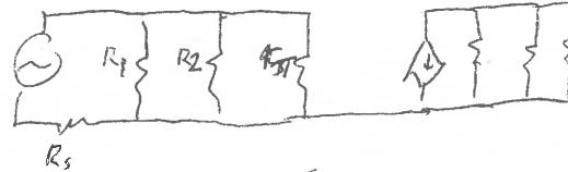
$$SCTC_{AC1} = C_{AC1} (R_1 || R_2) (r_\pi + R_S)$$
