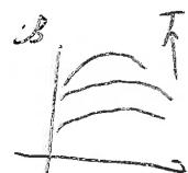
$\hookrightarrow$  To inject  $I_B$ , get  $I_C = \beta I_B$  ← linearly controlled
