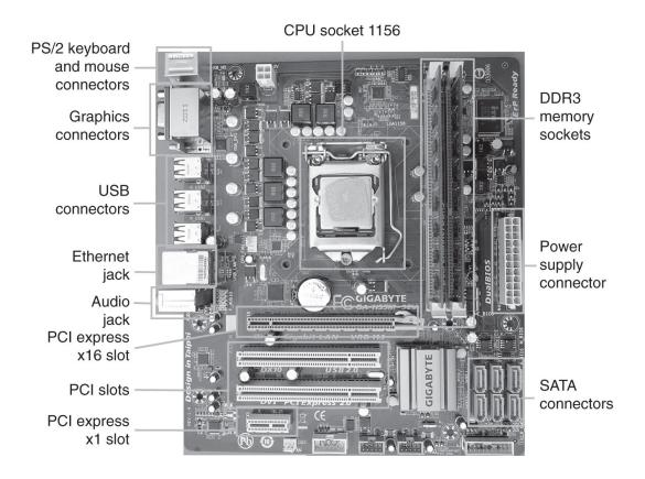
Figure 8.70 Gigabyte GA-H55M-S2V Motherboard
