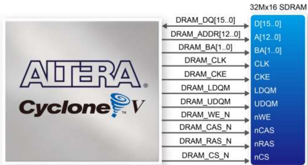
Figure 3-19 Connections between the FPGA and SDRAM
