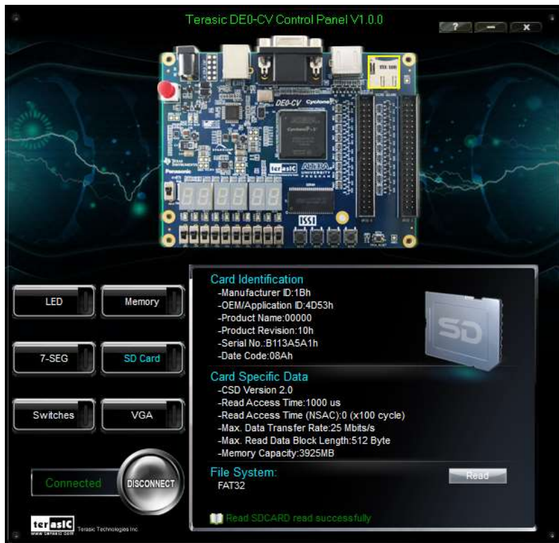
Figure 2-7 Reading the SD Card Identification and Specification
