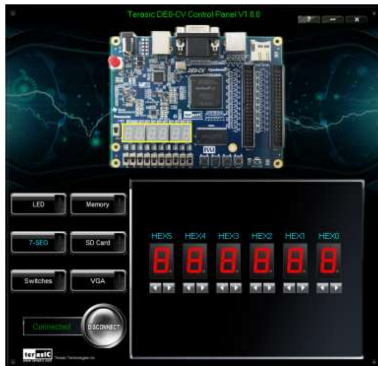
Figure 2-4 Controlling 7-SEG display
