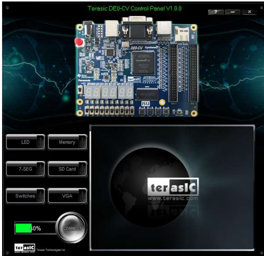
Figure 2-1 The DE0-CV Control Panel
