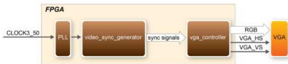
Figure 5-11 Block diagram of the VGA Pattern demonstration
