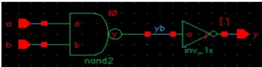
Figure 5: *and2* schematic
