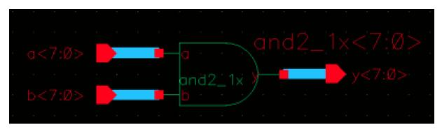
First instantiate an and  $2_1x$  from muddlib11. Choose Edit • Properties • Object... and change the Instance Name to and  $2_1x<7:0>$  to create 8 copies. Create the input pins (a<7:0> and b<7:0>) and output pins (y<7:0>). Choose Add • Wire (wide) and draw busses between the pins and the gate. Check and save and ensure you have no errors.
